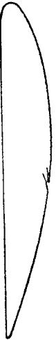
NACA 84-M wing section. Slot width = 0.667% c Slot at 53.9% c from leading edge. Internal pressure 12 q higher than free-stream static pressure
